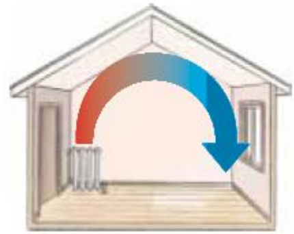
Figure 9.10: Convection currents are set up in a room heated by a radiator.
