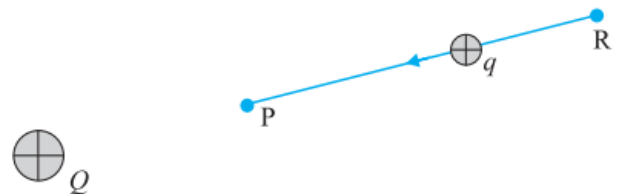
Figure 3.1: Electric field at test charge ( +q ) due to a charge ( +Q )
