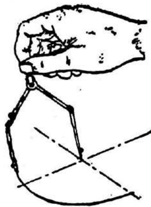
Fig.1.3 using the compass in drawing
