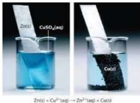
Figure 5. 6 The redox reaction of zinc metal with aqueous
