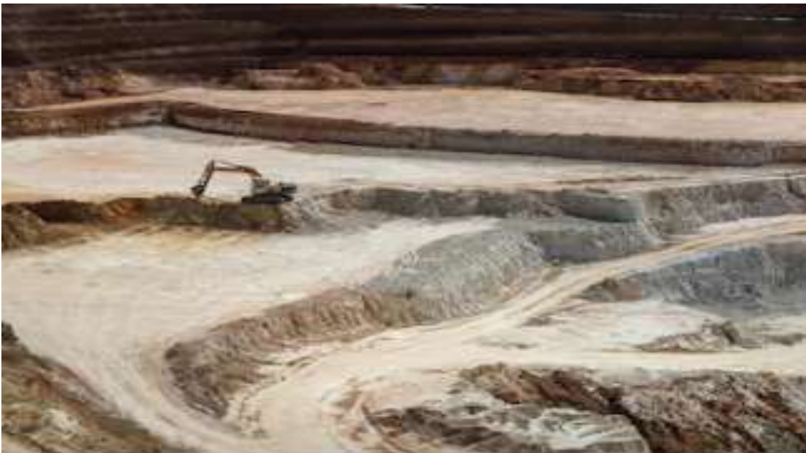
Figure 7. 6 Clays are excavated from open cast mines
