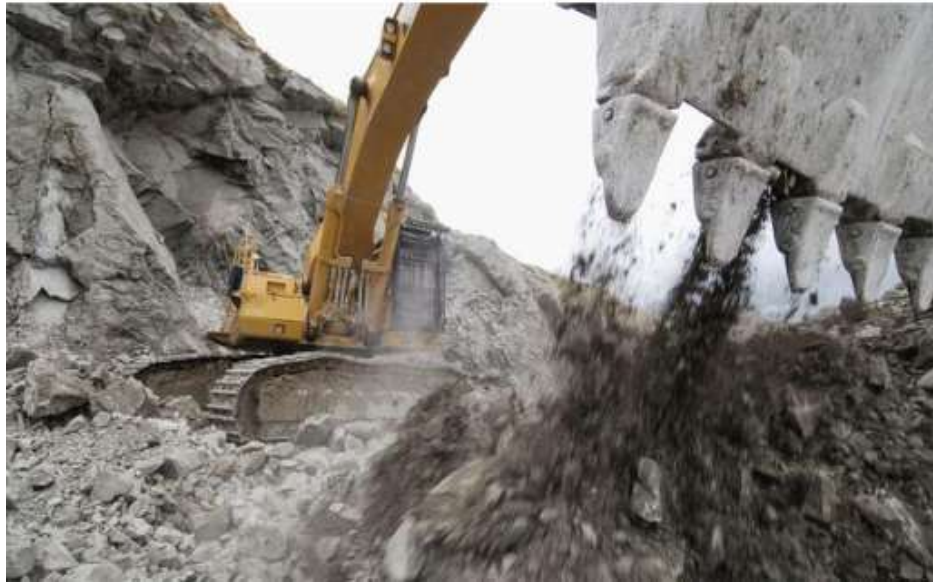
Figure 7. 4 Extracting raw material from quarry for cement manufacturing
